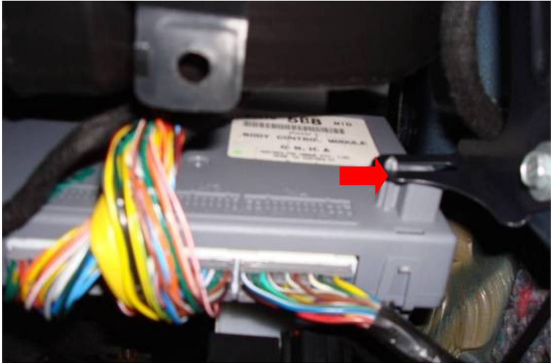
There is a scrivet where the arrow is, remove that and remove the wires that go into the BCM (you squeeze in the middle of the plugs to remove them).
