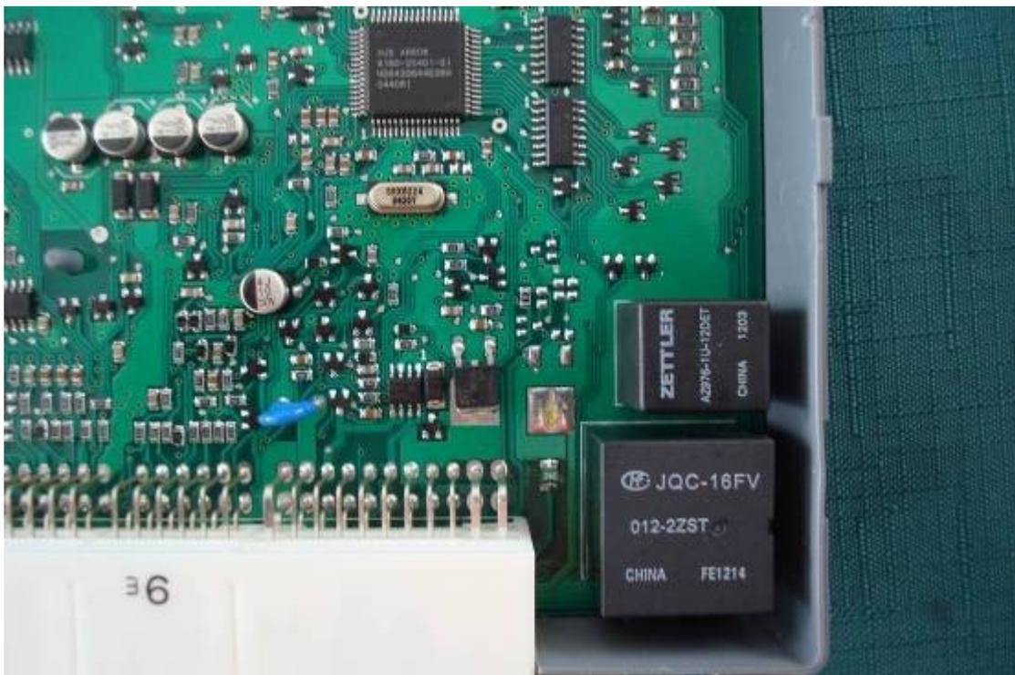
Solder the new relay in and reassemble everything and re-attach the battery. You should now have a working relay in there that will not stick and leave the indicator on when you lock or unlock your car.
