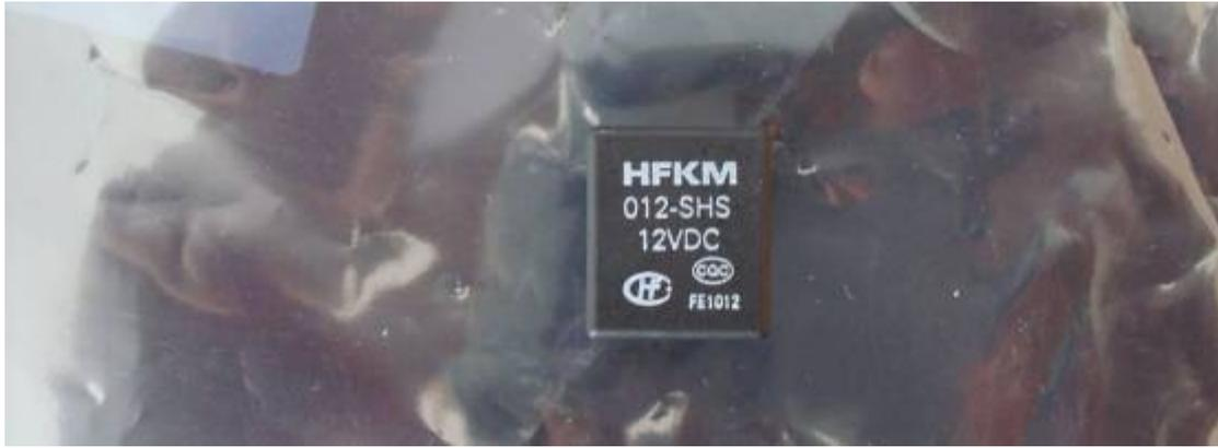
I replaced the relay with a Zettler AZ976-1U-12DET which a direct replacement for the HFKM-012-SHS relay.
