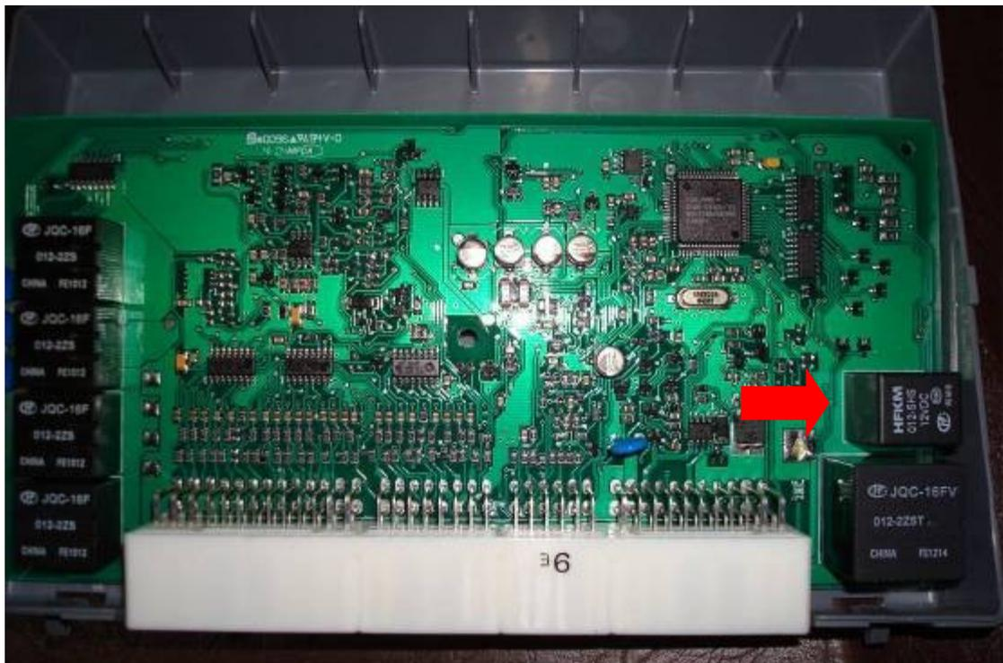
This is the relay that is sticking and causing the indicator to stay on. We will need to remove the relay and replace it.
